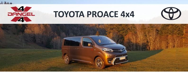
The PROACE 4x4 Dangel is the ideal solution for **safe driving in difficult conditions**: as soon as the front wheels lose their grip, the 4x4 system distributes part of the available torque to the rear wheels, allowing the vehicle to continue driving. This operation is carried out instantly, **without any intervention from the driver.**
