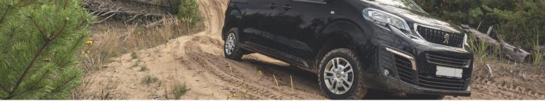
The EXPERT 4x4 Dangel is the ideal solution for **safe driving in difficult conditions**: as soon as the front wheels lose their grip, the 4x4 system distributes part of the available torque to the rear axle, allowing the vehicle to continue driving. This operation is carried out instantly, **without any intervention from the driver.**
