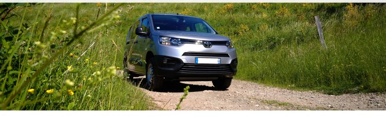
The PROACE CITY 4x4 Dangel is the ideal solution for **safe driving in difficult conditions**: as soon as the front wheels lose their grip, the 4x4 system distributes part of the available torque to the rear wheels, allowing the vehicle to continue driving. This operation is carried out instantly, **without any intervention from the driver.**
