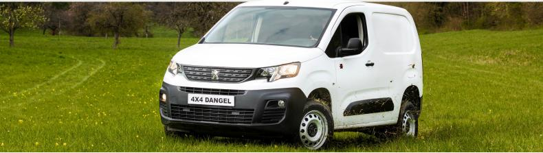
The PARTNER 4x4 Dangel is the ideal solution for **safe driving in difficult conditions**: as soon as the front wheels lose their grip, the 4x4 system distributes part of the available torque to the rear axle, allowing the vehicle to continue driving. This operation is carried out instantly, **without any intervention from the driver.**
