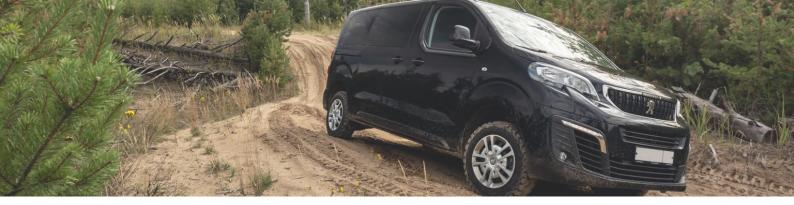
The EXPERT 4x4 Dangel is the ideal solution for **safe driving in difficult conditions**: as soon as the front wheels lose their grip, the 4x4 system distributes part of the available torque to the rear axle, allowing the vehicle to continue driving. This operation is carried out instantly, **without any intervention from the driver.**
