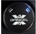
**AUTO 4WD Mode**: In conditions of normal surface grip, the vehicle work in front wheel drive, like the standard 2WD version. If the front axle loses
