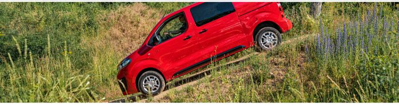
The VIVARO 4x4 Dangel is the ideal solution for **safe driving in difficult conditions**: as soon as the front wheels lose their grip, the 4x4 system distributes part of the available torque to the rear axle, allowing the vehicle to continue driving. This operation is carried out instantly, **without any intervention from the driver.**
