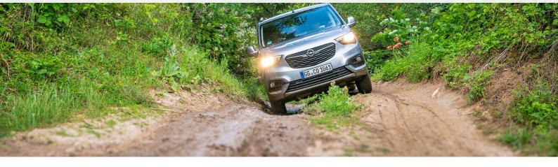
The COMBO 4x4 Dangel is the ideal solution for **safe driving in difficult conditions**: as soon as the front wheels lose their grip, the 4x4 system distributes part of the available power to the rear wheels, enabling the vehicle to continue driving. This operation is carried out instantly, **without any intervention from the driver.**
