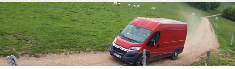
The JUMPER 4x4 Dangel is the ideal solution for **safe driving in difficult conditions**: as soon as the front wheels lose their grip, the 4x4 system distributes part of the available power to the rear wheels, enabling the vehicle to continue driving. This operation is carried out instantly, **without any intervention from the driver.**
