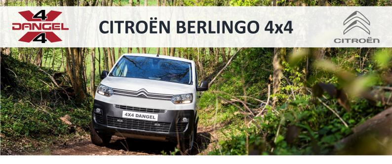
The BERLINGO 4x4 Dangel is the ideal solution for **safe driving in difficult conditions**: as soon as the front wheels lose their grip, the 4x4 system distributes part of the available torque to the rear axle, allowing the vehicle to continue driving. This operation is carried out instantly, **without any intervention from the driver.**
