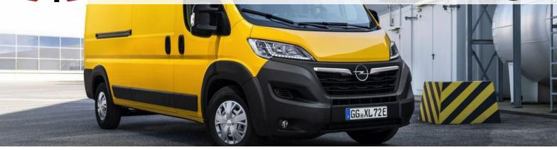
THE MOVANO 4x4 Dangel is the ideal solution for **driving safely in difficult conditions**: as soon as the front wheels lose their grip, the viscocoupler distributes part of the available torque to the rear axle, allowing the vehicle to continue driving. **This operation is carried out instantly, without any intervention by the driver**.
