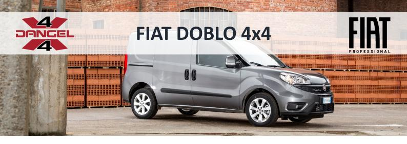
The DOBLO 4x4 Dangel is the ideal solution for **safe driving in difficult conditions**: as soon as the front wheels lose their grip, the 4x4 system distributes part of the available power to the rear wheels, enabling the vehicle to continue driving. This operation is carried out instantly, **without any intervention from the driver.**
